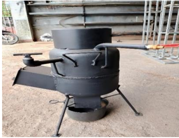
Figure 1. Overfire-Injection Biomass Stove Used in The Experiment
